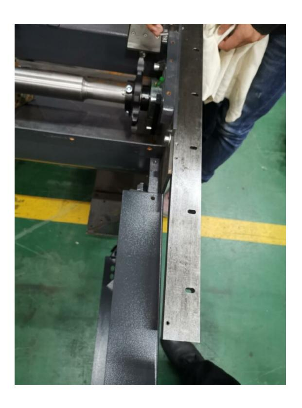
2. Install the height adjustment block from the second mounting hole (the baffle slope).
