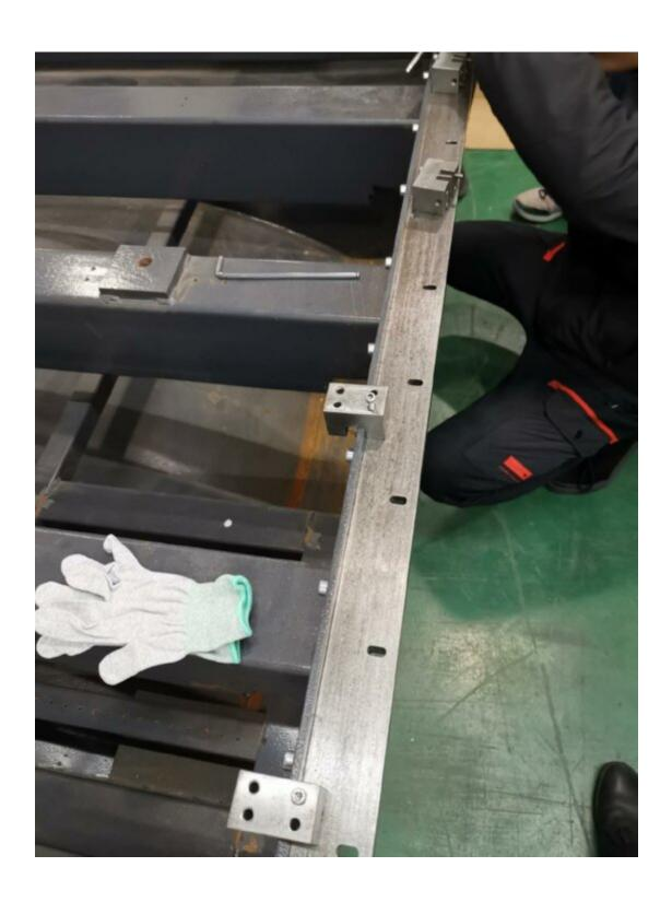
2. Adjust the height to 15mm, the figure below shows that the value is higher than 15mm, you need to tighten the bolt on the height adjustment block to adjust.
