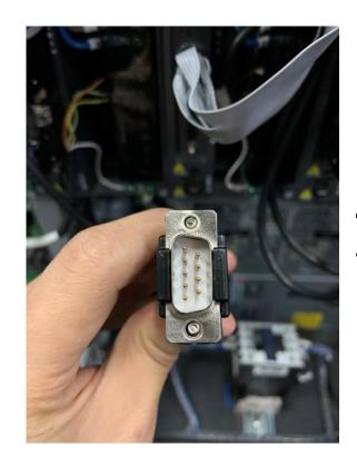
1.Find the 4,5,7,8 pins in the encode cable plug
