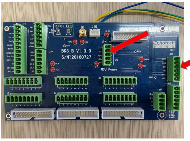
If the power input is good but the voltage of the DRT/PRT is not correct, it means your B board is broken.
