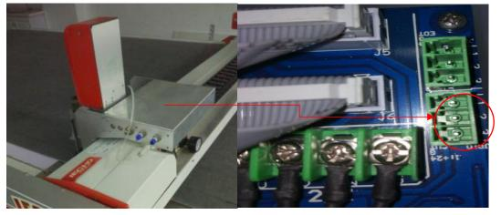
**2.** If the voltage is correct, check the DRT/PRT cable communication. If the cable communication is good, mean your DRT/PRT is broken.
