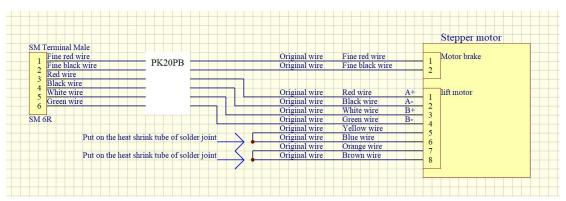
Result of reason1: Motor running is shaky, and throw the step; The motor brake does not work, resulting in the motor shaft running with the brake, resulting in too much noise.
