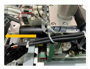
3. Unlock the four screws and the middle one, then take off the motor.
