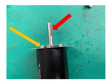
5. Unlock the four screws, then remove the old motor. There is a flat surface on the pole, which is used to lock it by fastening nails when the motor is mounted on another part
