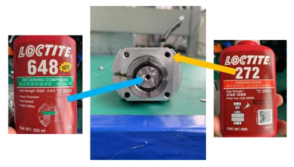
7. Then lock the screws back, using 272 and 648 glue. Please make it sure all the screws are tightened.
