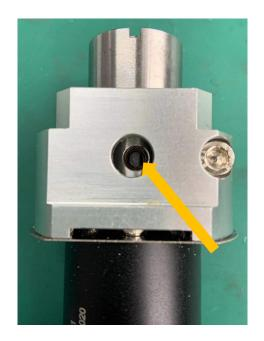
4. Unlock the four screws as well as the internal tight nail to separate the motor. About the tight nail, you can rotate the rotate the pole on the motor to find it.
