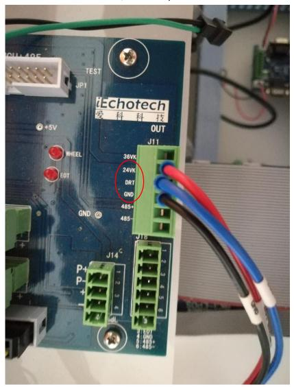
**2.** If the voltage is correct, check the DRT/PRT cable connection. If the cable connection is good, it means your DRT/PRT is broken.
