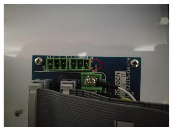
**3.** If the DRT/PRT always rotates, check the blue and black cables in DRT/PRT plug on the B board. When DRT/PRT tool isn't selected in the software, the voltage should be zero. If not, it means your B board is broken.
