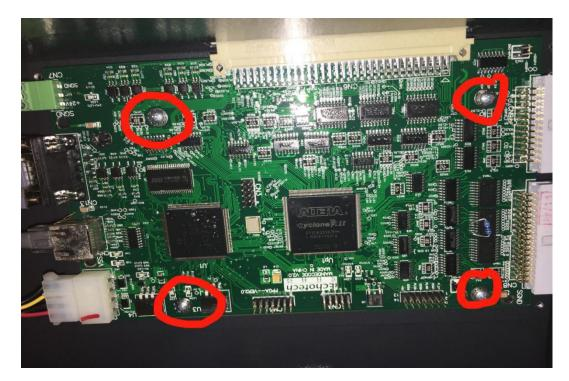
4. Remove the clamping screws of the DSP board.
