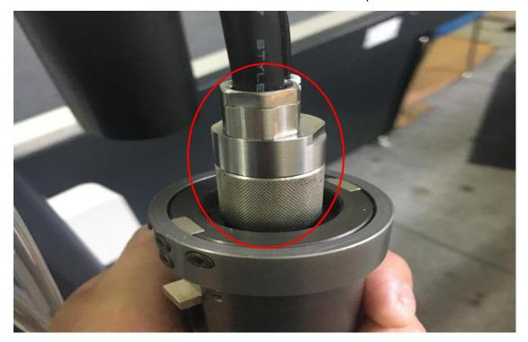
Check if the router cable connector fixed to the end on E3000 driver.
